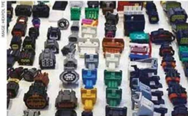
**Above: Hexpol TPE has developed materials for adhesion to polyketone substrates during multi-component injection moulding**
